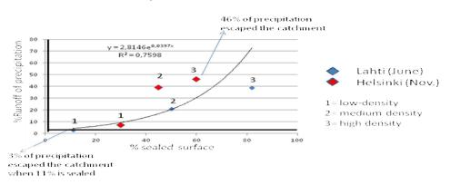
How much of the rain flows out of the catchment in relation to % impevious soil surface
